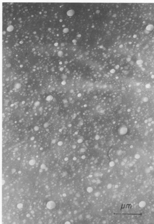
Figure 5 Transmission electron micrograph of an ultra-thin layer of the composite formed in a type 3 reaction
